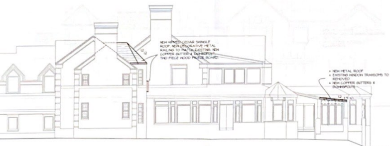
EXISTING/DEMO SOUTH ELEVATION 1/8" = 1'-0"
