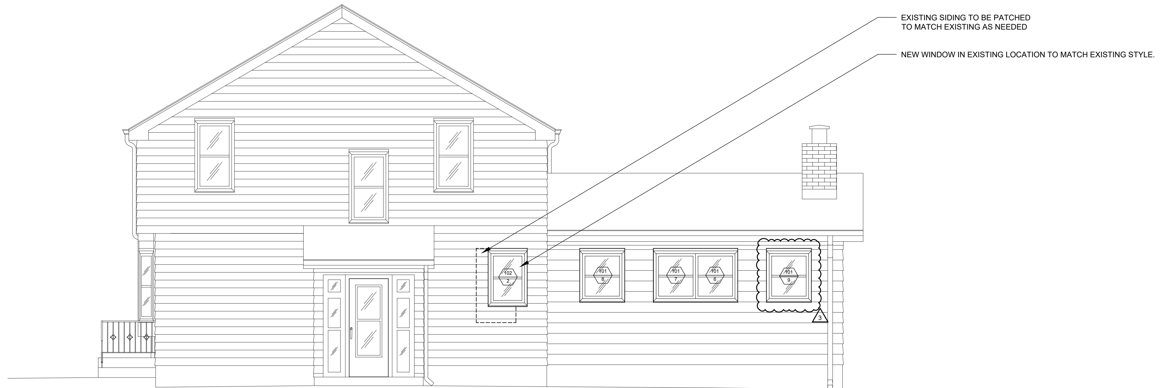
2 NORTH ELEVATION - PROPOSED SCALE: 1/4" = 1'-0"
