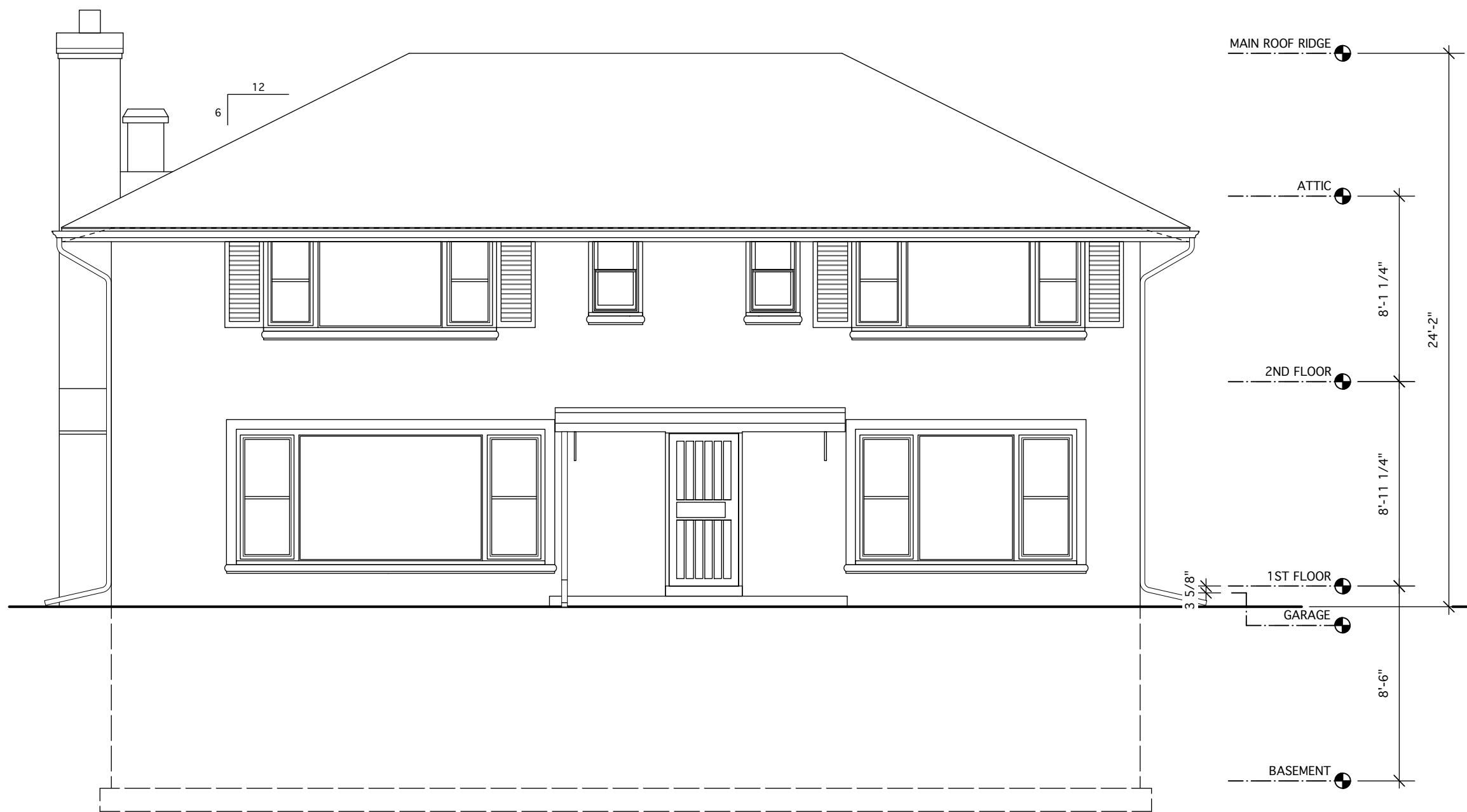
1 EXISTING/DEMOLITION FRONT/WEST ELEVATION Scale: 3/16" = 1'-0"
