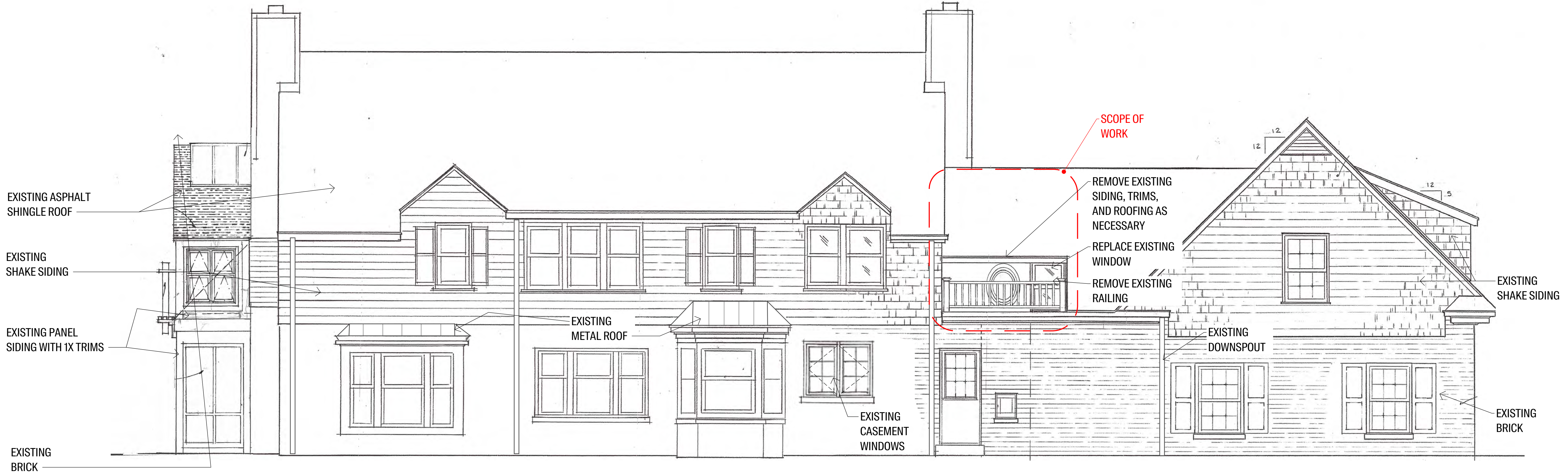
1 A-4 Existing East Elevation 1/4" = 1'-0"
