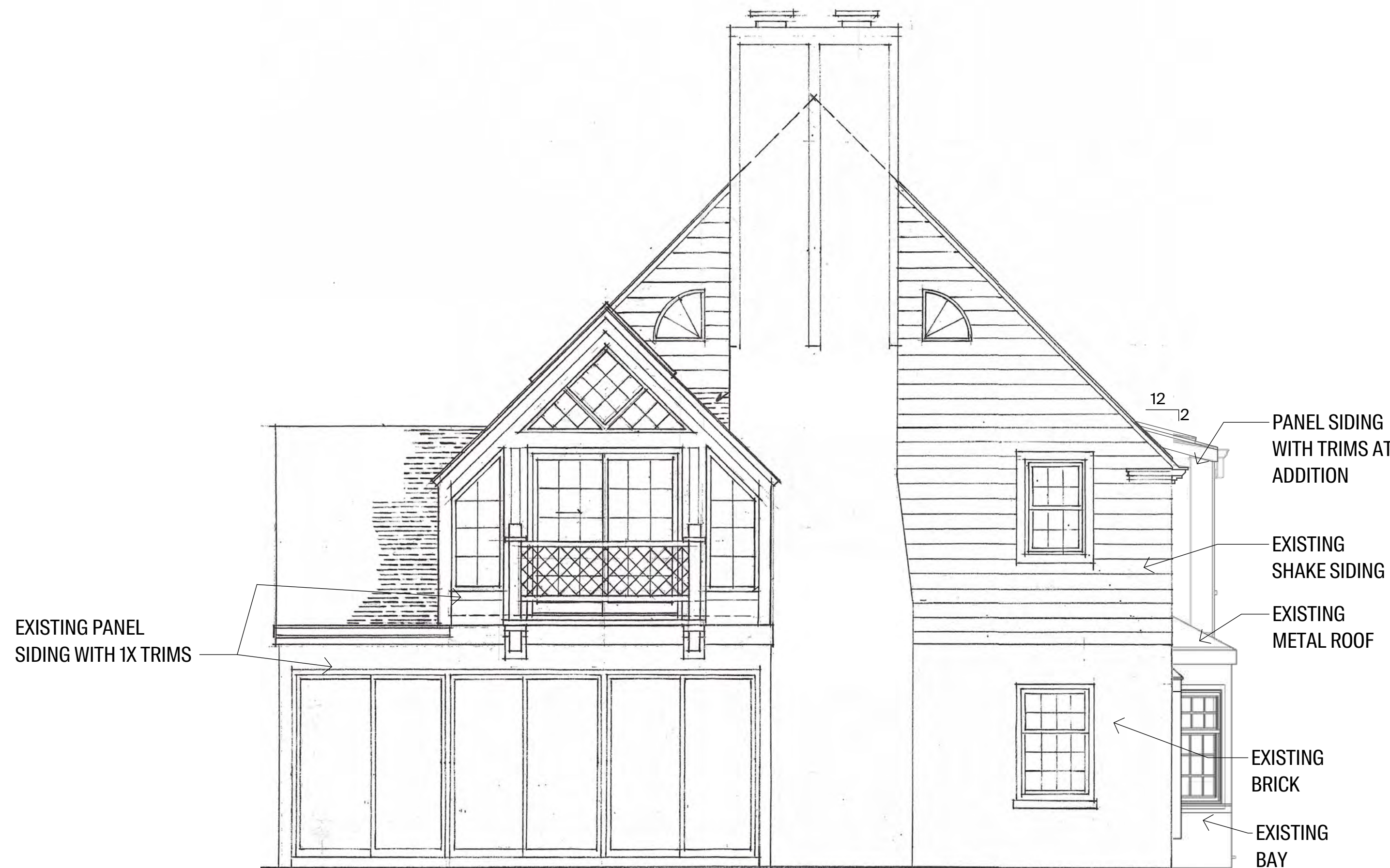
3 A-5 Existing South Elevation 1/4" = 1'-0"
