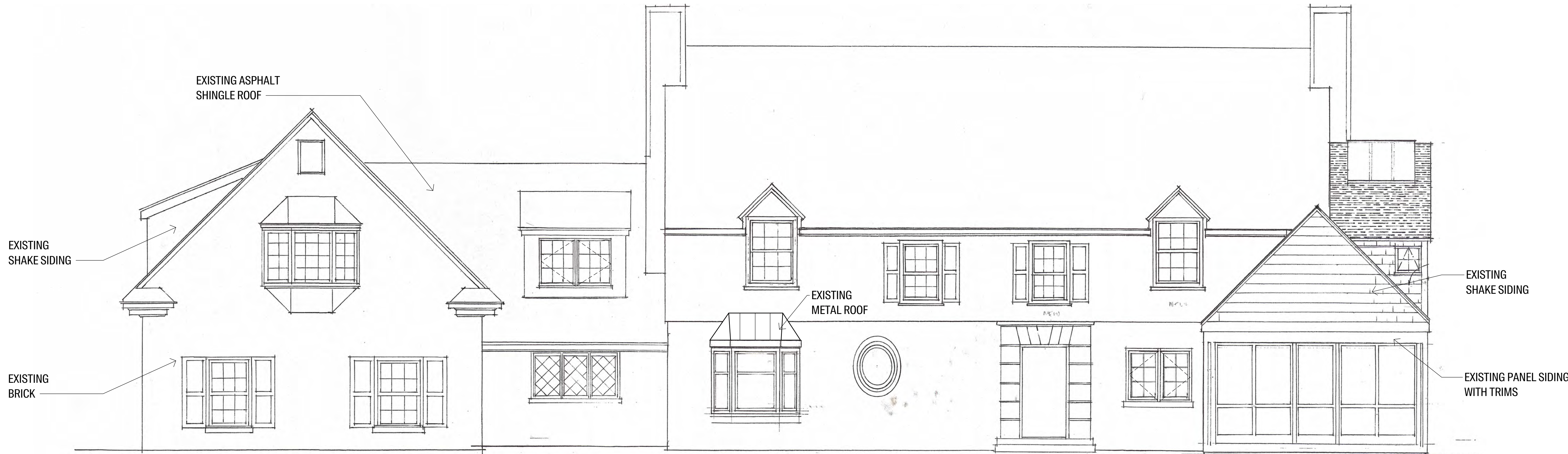
1 A-5 Existing West Elevation 1/4" = 1'-0"
