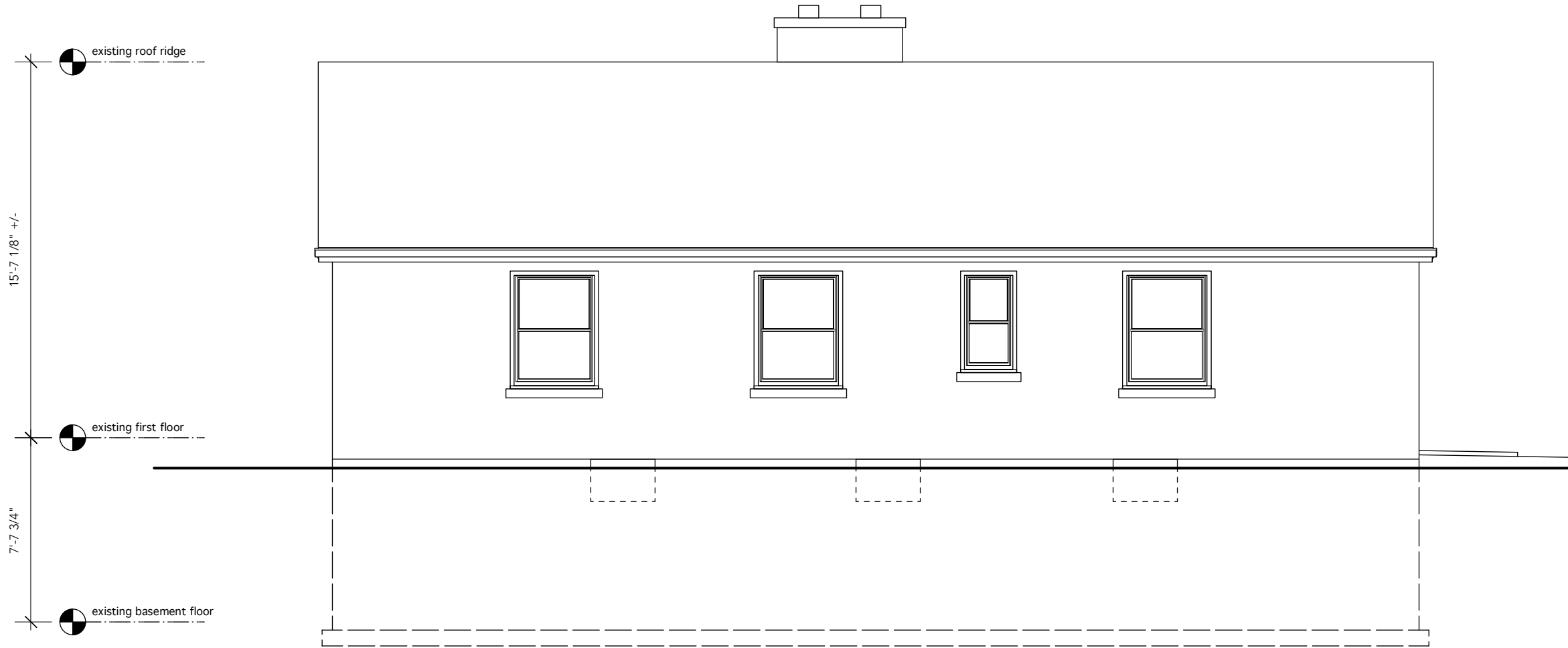
5 EXISTING/DEMOLITION REAR/WEST EXTERIOR ELEVATION D101 SCALE: 3/16" = 1'-0"
