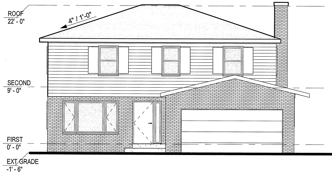
2 WEST (FRONT) ELEVATION - EXISTING 1/8" = 1'-0"
