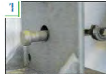
1 Install the bolt into the hole followed by the collapsible washer.
