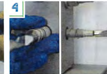
4 Engage the spring shear sleeve into the shear plane.
