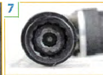
7 Using the shear wrench engage the outer socket with the splined end of the bolt. Press the trigger until correct tension has been achieved (the bolt spline separates from the bolt).
